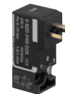
Directional control valve, D016 series Qn = 16 – 25 l/min. Electr. connection: plug, ISO 15217, form C
