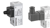
Pressure switch, PM1 series Switching pressure: -0.9 – 16 bar, electr. connection: plug, ISO 4400, form A and M12x1, 4-pin
